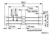
Minimum lead spacing 10 mm
